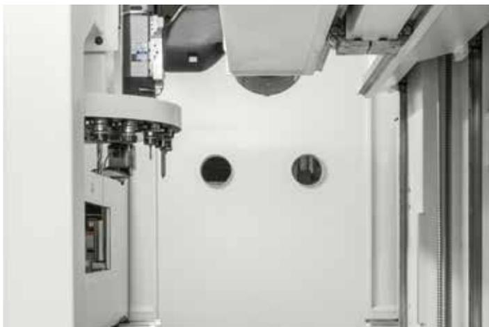
**Elimination of dust.** Suction outlets are placed on the perimeter of the cabin, in order to collect the finest dust and keep the work area always clearly visible.
