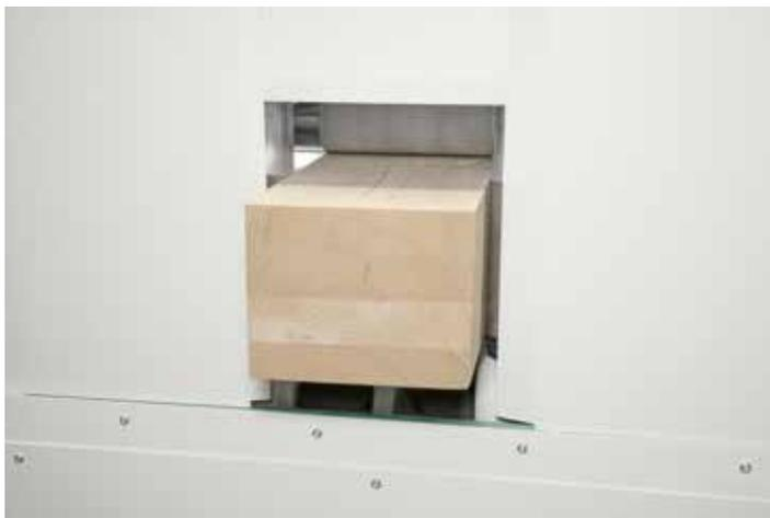
**Dust containment.** The motorized casings surrounding the beam infeed and outfeed of the work area determine dust and shavings containment inside the cabin.
