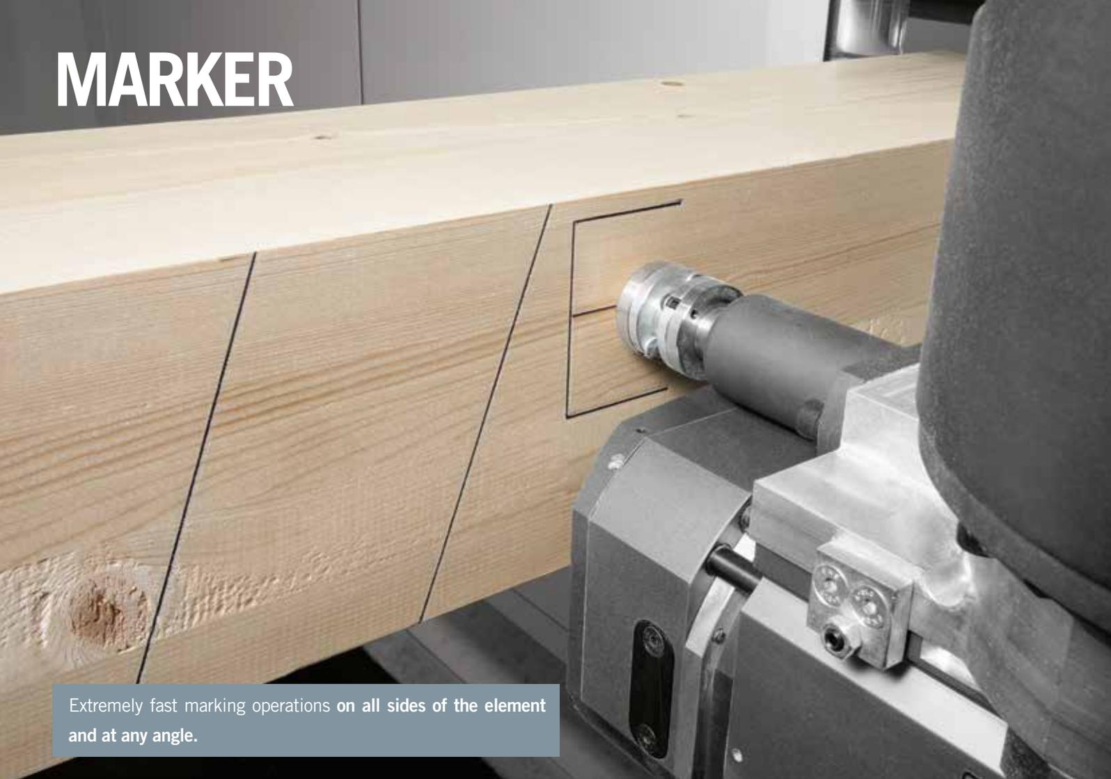
Extremely fast marking operations **on all sides of the element and at any angle.**
