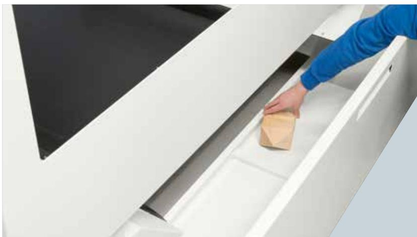
The operator can easily recover the short pieces through a special door positioned on the front of the cabin.
