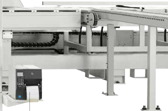
**Simple identification** of each element thanks to "label printing" at the end of processing.
