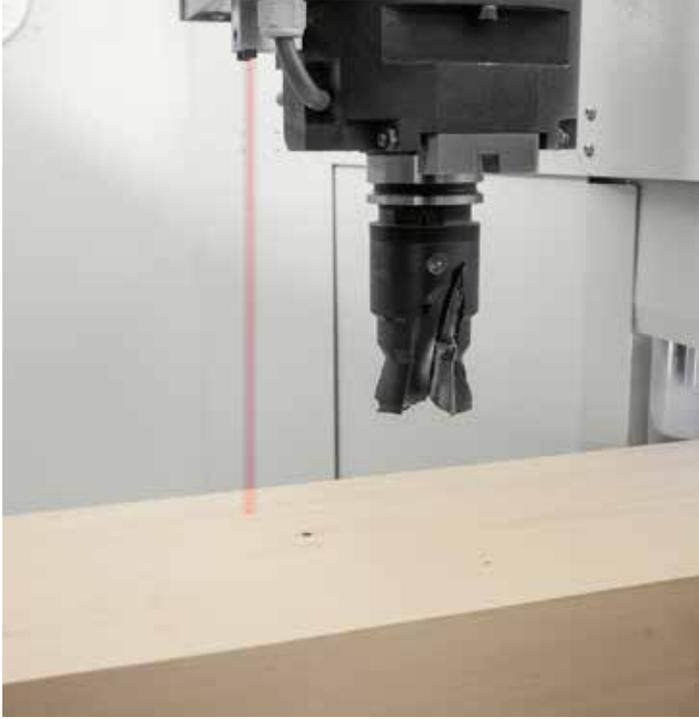
Laser probe detects the exact position on the element side where operation must be performed, to guarantee high accuracy.
