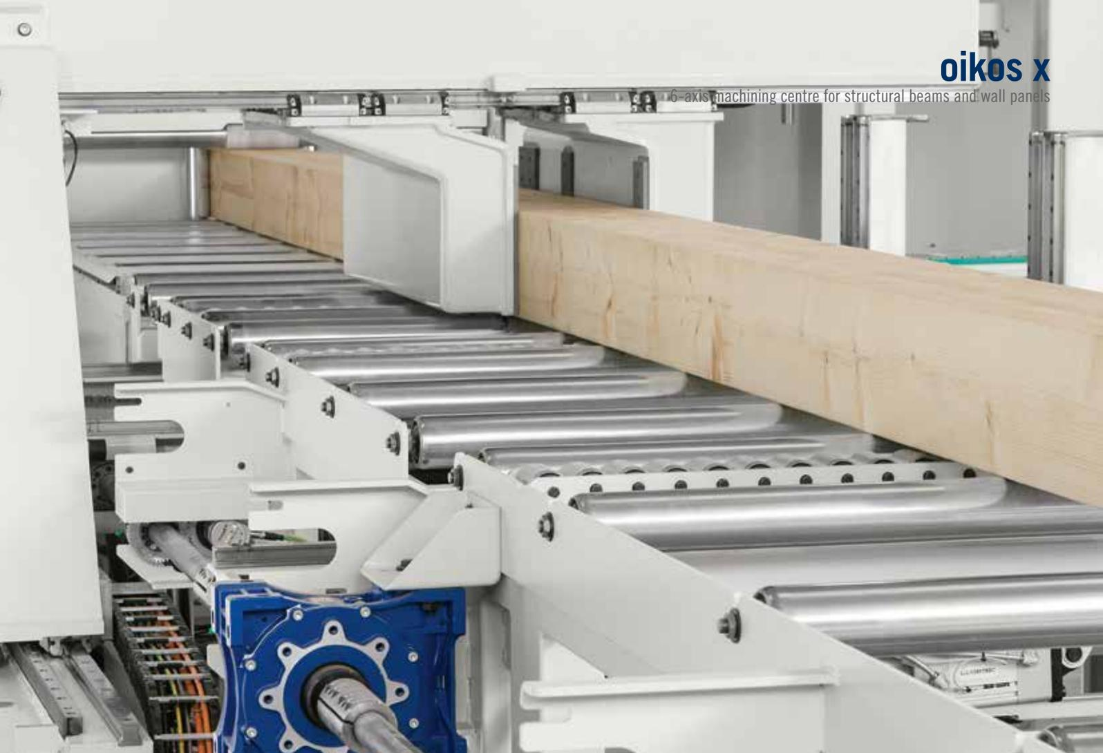
The element is locked and moved along the longitudinal axis by a carriage equipped with a clamp that ensures optimal grip in all conditions. The jaws of the clamp are self-centering hence the beam is always aligned to the centre of the loading roller conveyor.
