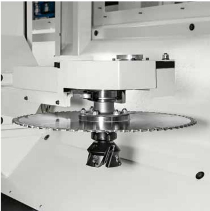
Made up of a support fully compatible with the electrospindle and with the tool stations inside the cabin, the “integrated tool” can host a 440 mm diameter sawblade and a cutter at the same time for making slots and pockets.
