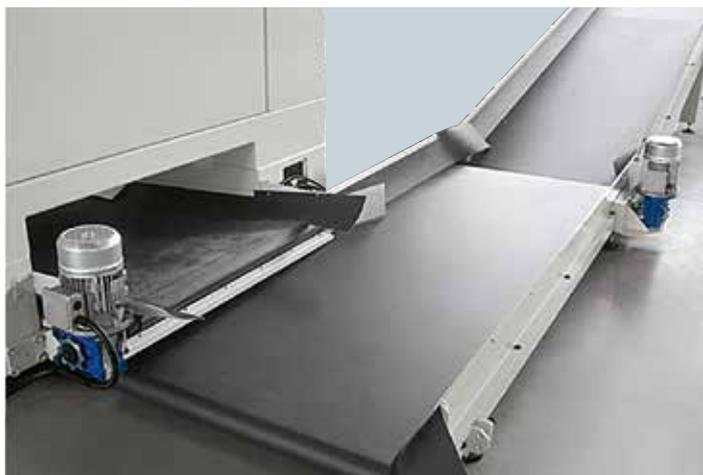
**Always clean work area.** An inclined rear conveyor belt connected directly to a container collects shavings and waste.
