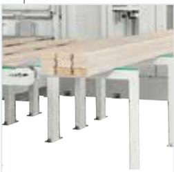
*Easily extractable supports to place packages of beams in front of the loading chains.*
