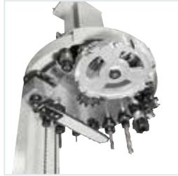
Rapid 15 tool store positioned near the work area **to reduce tool change time.**
