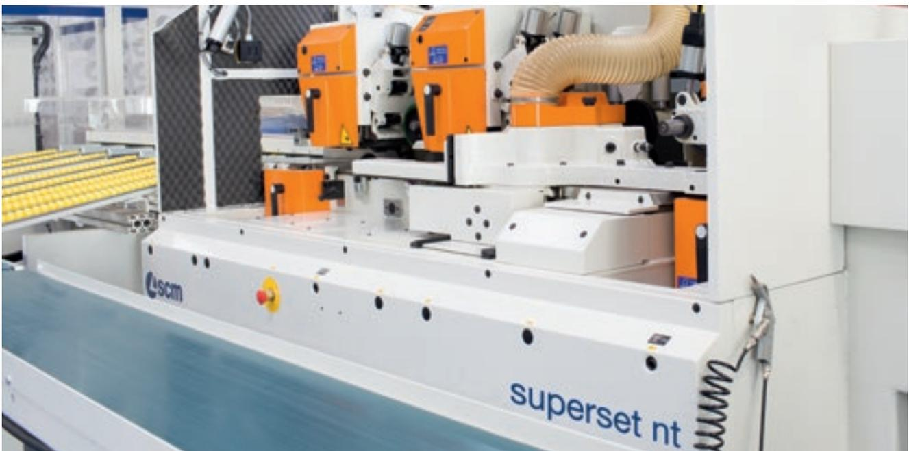
Work piece return system to the operator.
