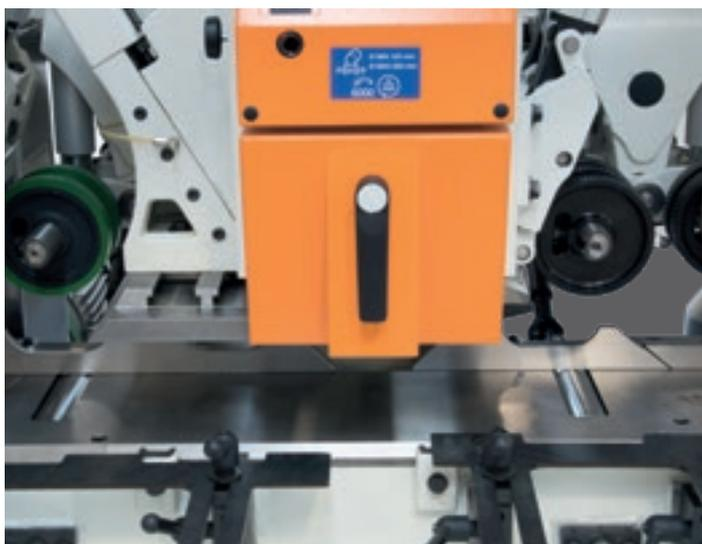
Possibility to supply 2 rollers on the worktable, before and after the 1st upper horizontal spindle, for a uniform feeding of the workpiece in the machine.
