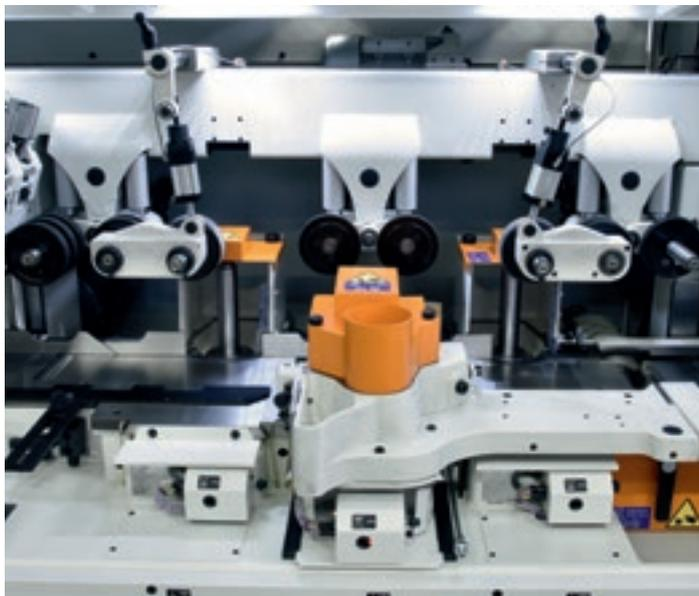
Also on the Superset NT range is available the **2nd right vertical spindle** in the compositions with two upper horizontal spindles, with and without the universal spindle.
