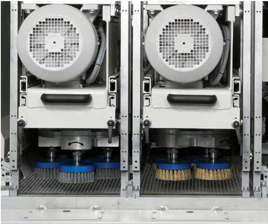
The sanding or structured effect on products with cross grain, such as for example cupboard doors or door and window frames, is achieved with the multi-directional sanding action of the **planetary units**.
