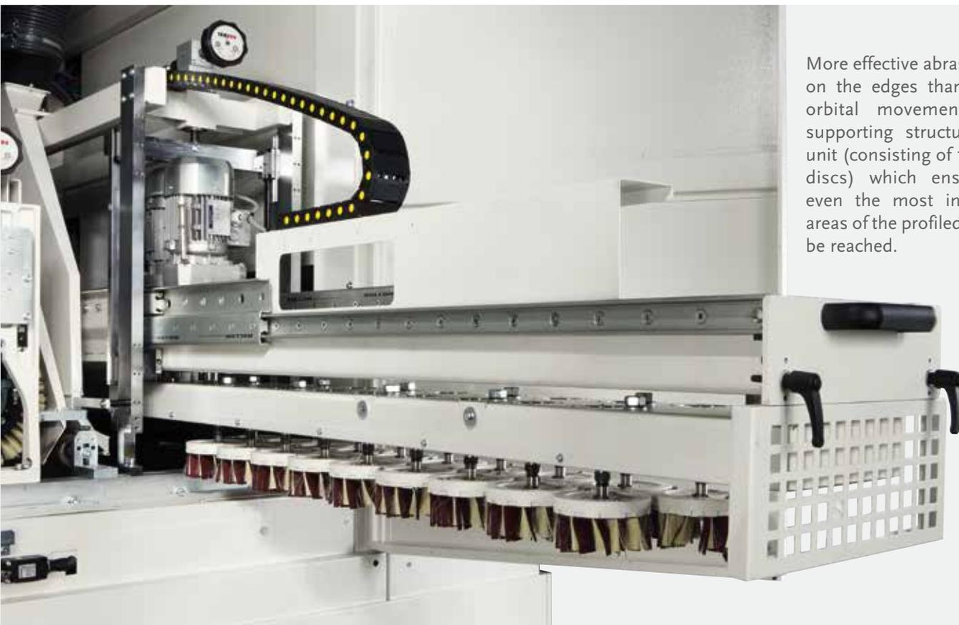
More effective abrasive action on the edges thanks to the orbital movement of the supporting structure of the unit (consisting of 19 rotating discs) which ensures that even the most inaccessible areas of the profiled panel can be reached.
