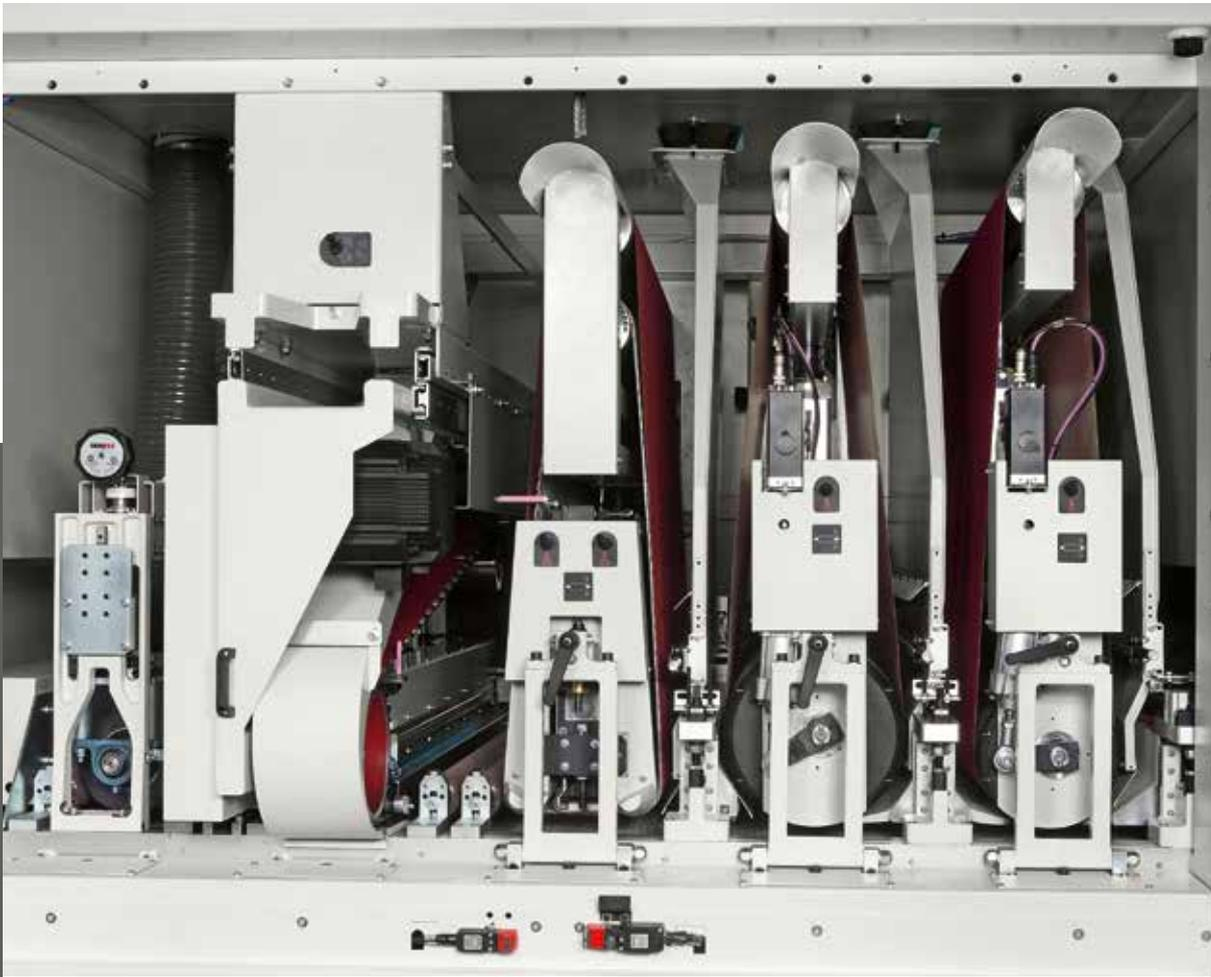
The configuration of the DMC System 1350 T5 shown here, fitted with calibration roller, large diameter sanding roller, superfinishing pad, crossbelt unit and satinising roller, fulfils all the production and finishing requirements of industrial companies and demanding contractors which need to combine productivity with flexibility.
