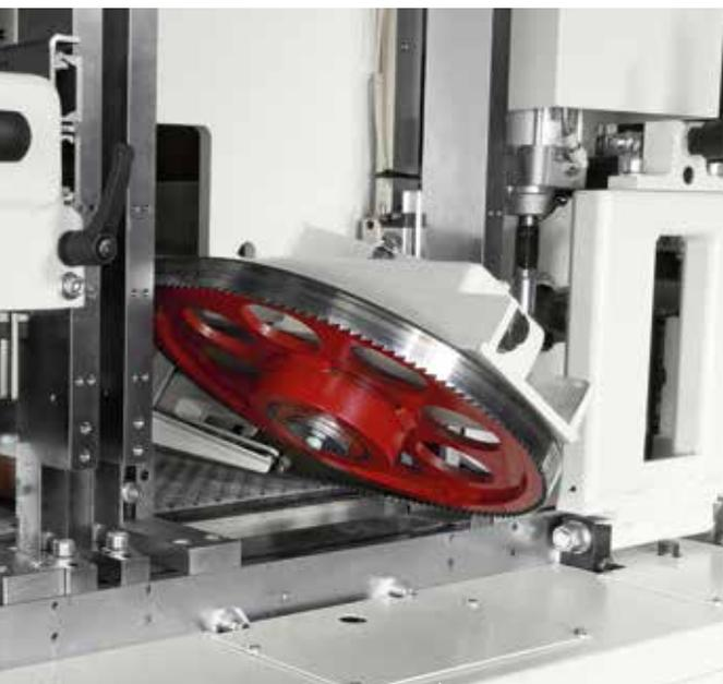
The innovative “**saw blade**” unit allows users to recreate the irregular surface effect produced by using a bandsaw. The ability to regulate the depth of the blade cut, and the rotation speed of the blade, enables the user to control the depth and distribution of the cuts, making it possible to choose the kind of finish users wish to create every single time.
