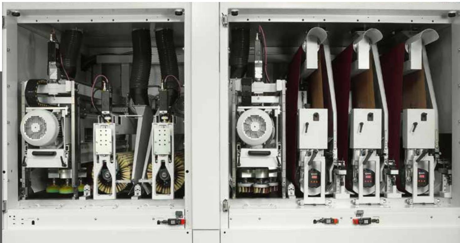
The DMC System T7 1350, which is fitted with 7 main operating units, is the most advanced solution currently available on the market to machine kitchen doors and window frames, both assembled and single parts. From the calibration straight to the superfinishing, in a single pass through the machine:
