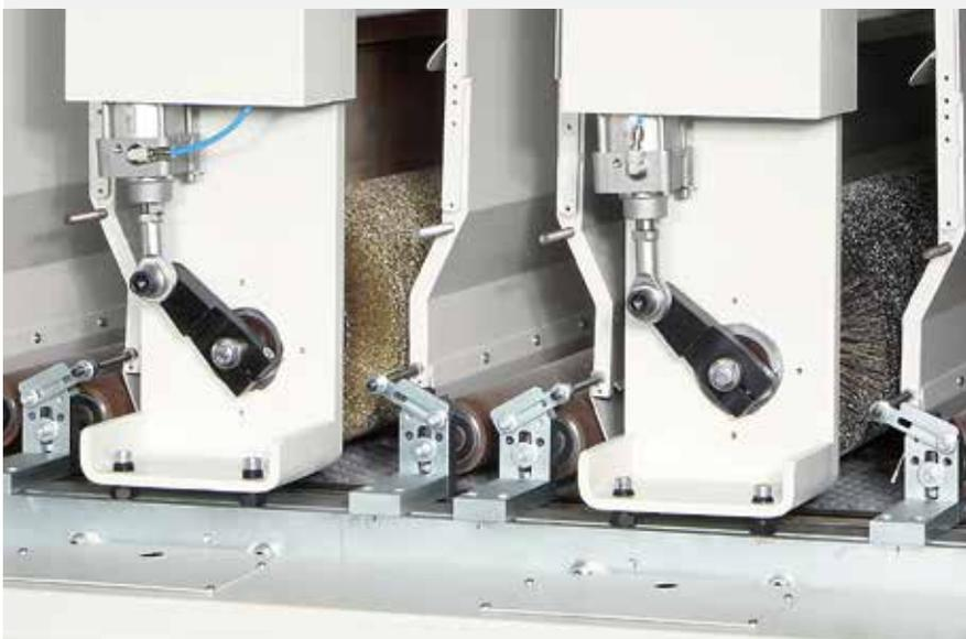
The **structuring roller** units allow to achieve finishing effects which range from a slight opening of the pores to extreme structuring. Perfect machining results are guaranteed thanks to the robust supporting structure and the power of the available motors.
