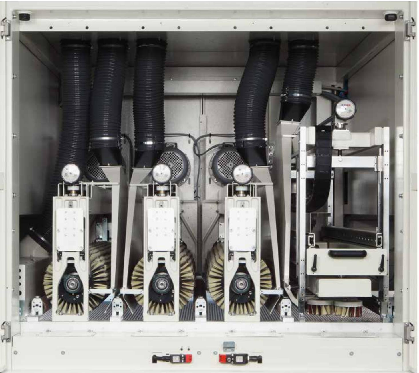
The ideal configuration for creating finishes for assembled doors, window frames and profiled elements in general (strips for frames, door and window frames, trims, matchboards, skirting boards, etc.), regardless of whether they are rough or painted.
