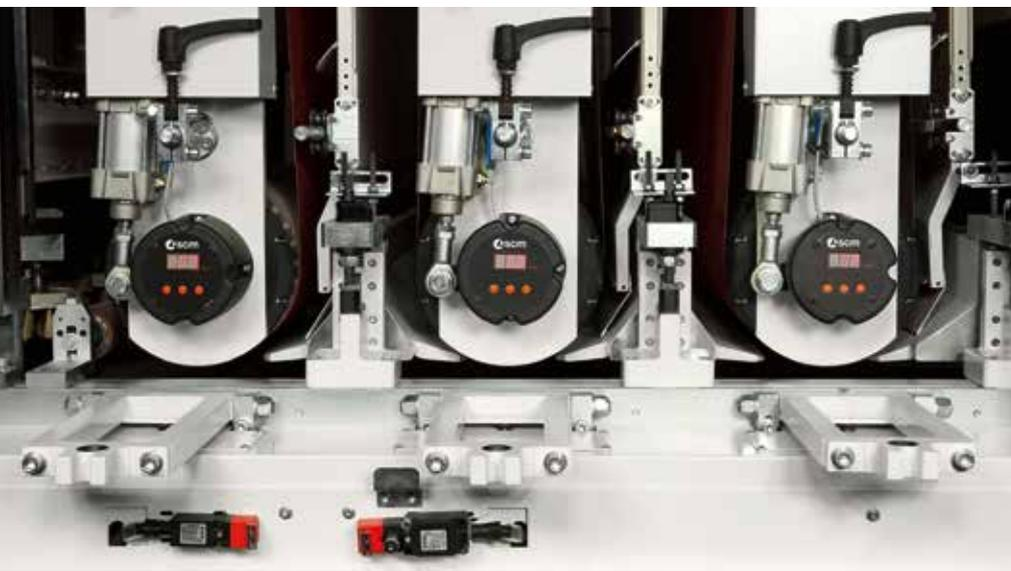
The DMC System T7 1350 contact rollers are equipped with heavy pressure bar units, fitted with a monolithic structure and vertical sliding prism guides: maximum precision and reliability in machining door and window frames and in calibrating with high stock removal.
