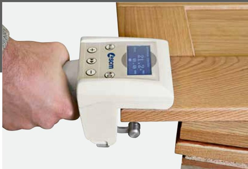
The wireless electronic gauge allows the machine to be positioned at the work thickness measured by the device. The communication with the machine is wireless and the working program can also be launched from the remote control.
