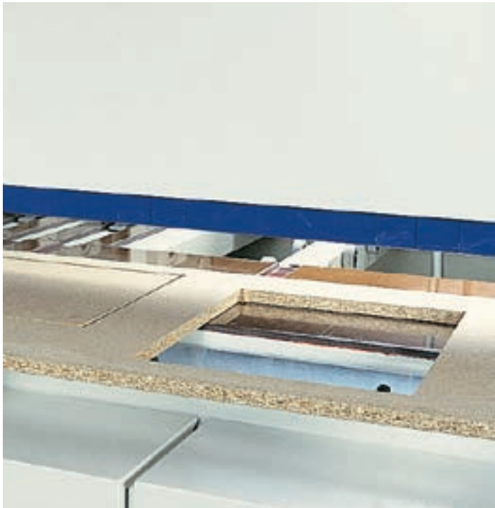
SLOTS EXECUTION DEVICE: AT THE OPERATOR'S SERVICE This device allows carrying out interrupted cuttings inside the panel to produce slotted doors (opt.).
