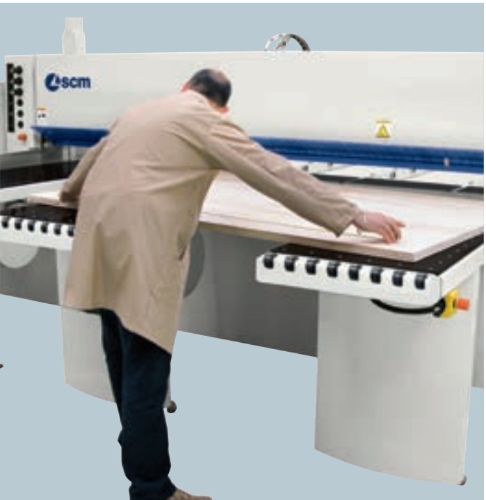
AUTOMATIC WORKPIECE MEASUREMENT: NO POSSIBILITY OF ERRORS The device automatically detects both the panel size and its position on the work table avoiding difficult manual operations in case of very long panels and slowing down in the production cycle (opt.).
