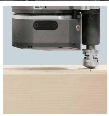
The pressurized ink pen is placed in a pneumatic device able to take it outside machining area if not in use.
