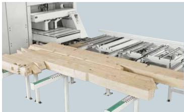
A pusher placed on the rear side of the unloading system moves the element onto an accumulation buffer.
