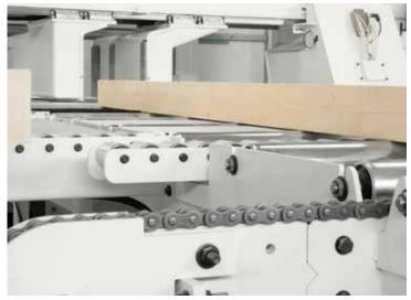
With standard positioning on the machine right side, the system manages processed elements unloading.
