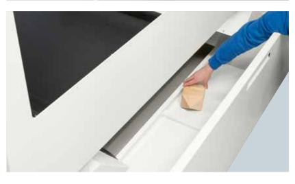
The operator can easily recover the short pieces through a special door positioned on the front of the cabin.
