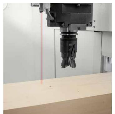
Laser probe detects the exact position on the element side where operation must be performed, to guarantee high accuracy.
