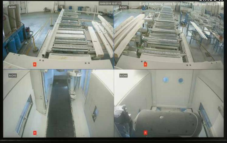
**Video surveillance system.** The video surveillance system allows the operator to monitor in real time the machine status through a monitor positioned above the eye-M console. Use of 4 high-resolution cameras.
