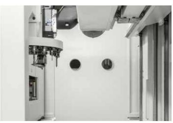
**Elimination of dust.** Suction outlets are placed on the perimeter of the cabin, in order to collect the finest dust and keep the work area always clearly visible.
