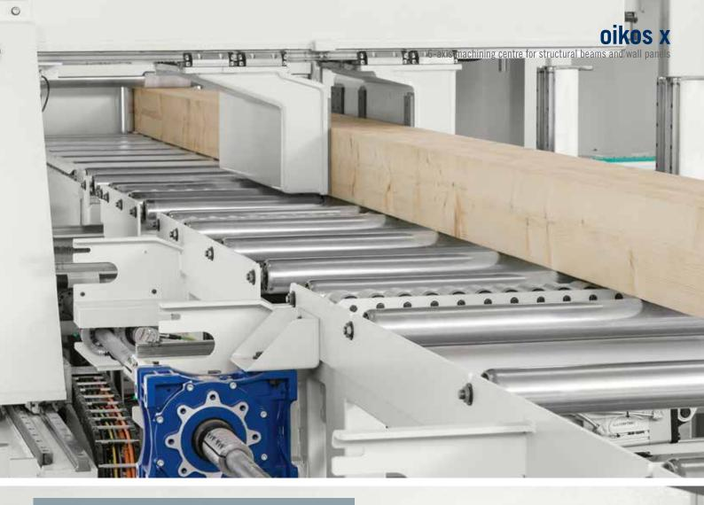
The element is locked and moved along the longitudinal axis by a carriage equipped with a clamp that ensures optimal grip in all conditions. The jaws of the clamp are self-centering hence the beam is always aligned to the centre of the loading roller conveyor.
