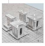
Worktable Available in phenolic multilayer or aluminium, it has an integrated vacuum system and grooves on the entire surface.
